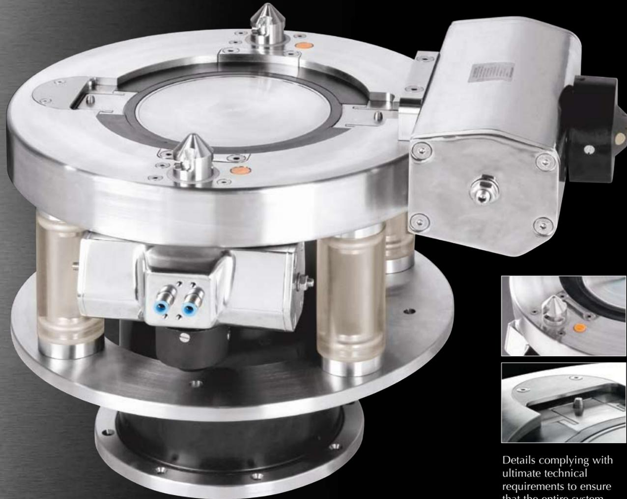
The docking process can be achieved either with a mobile container using a lifting column, or automatically with lifting cylinders mounted directly on to the active valve. After undocking, the active valve will return to its centred position. When redocking, the active valve will pinpoint the passive valve with an accuracy of  $\pm 14$  mm.
