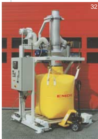
Compact filling station, removal of the full bags by manual pallet truck
