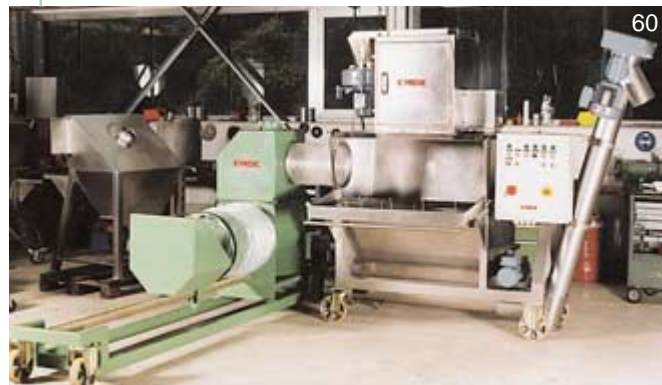
Mobile EMDE empty bag compactor at a sack emptying station
