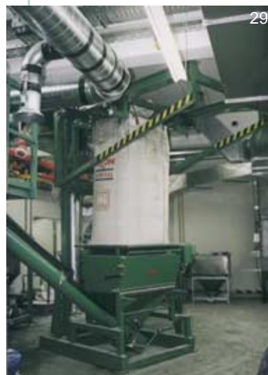
Combined sack and FIBC discharger
