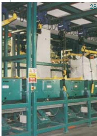
Multi-component dosing plant for the production of abrasives
