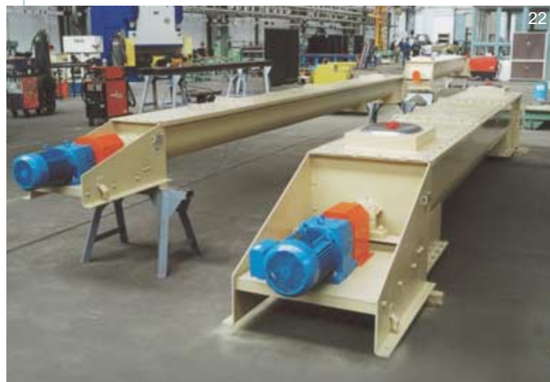
WUTRA trough screw conveyor for the transport of wood chips
