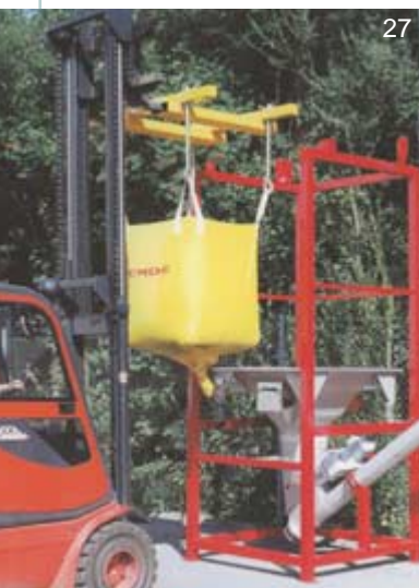
Loading the discharge station using a fork truck
