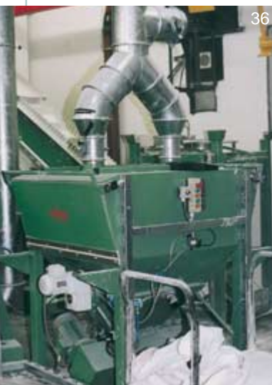
EMDE sack discharger for use with additives
