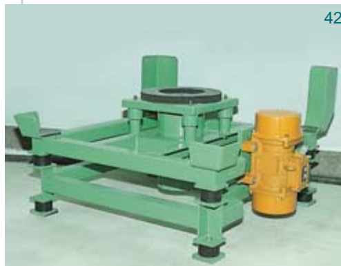
EMDE IBC discharger with vibratory discharge aid
