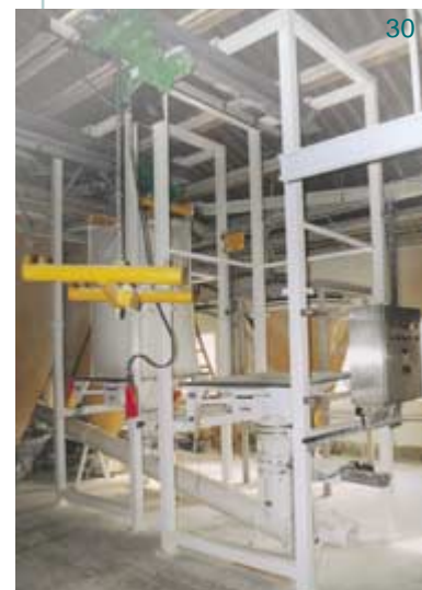
EMDE FIBC discharger with lifting device for the food industry
