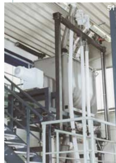
EMDE double-screw mixer as a weighing bin
