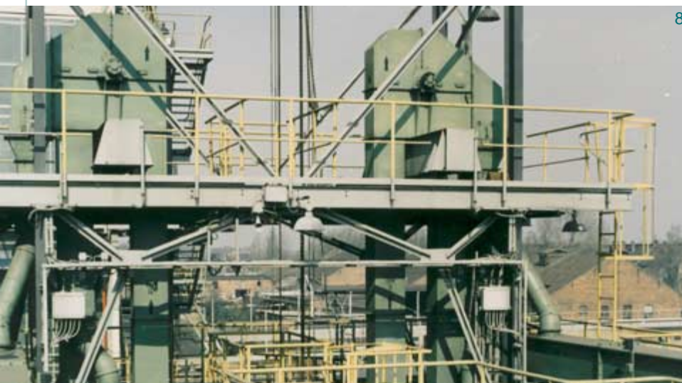
Grain handling with WUTRA belt type bucket elevators
