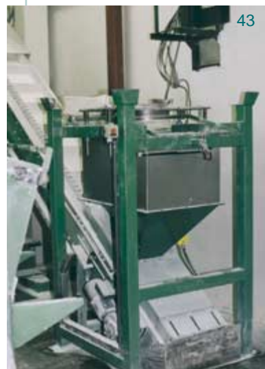
IBC discharger feeding a belt conveyor
