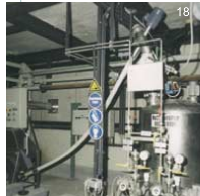
Feeding a batch vessel with EMDE-LIFT
