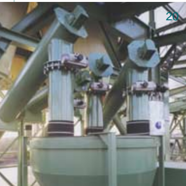
WUTRA tubular screw conveyor for multi-component dosing
