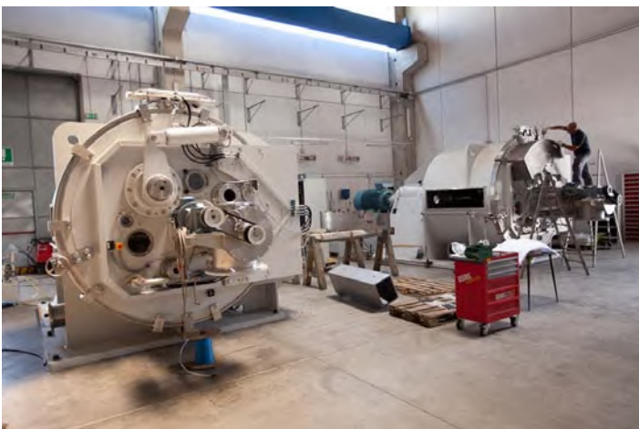
Peeler model HX/S/L 2000/1400 in a large starch production plant
