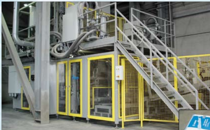
Nett weighing and screw dosing system for cement and cement based mixtures. The system produces water/weather proof bags by using 'non perforated' tubular film and a vacuum chamber incorporated in the closing section.
