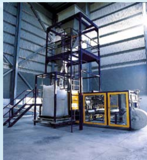
The nett weighing principal can be used to fill big-bags as well as sacks.
