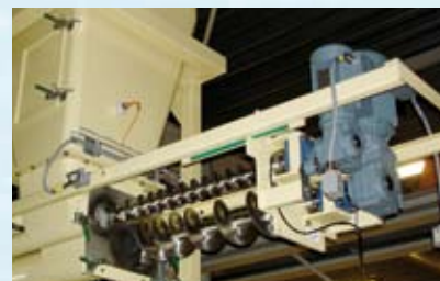
Removable dosing screws providing optimal access for cleaning.
