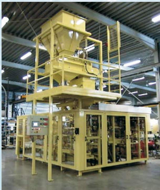
Nett weighing system with duplex weighing and belt conveyor dosing - pet-food. Designed as a "combi-system" the system is suitable for handling pre-made sacks as well as processing them drawn from the reel. A range of closing devices, such as heat sealing, stitching or pinch, are available that can be selected individually or in combination.
