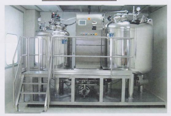
Preparation and storage systems for batches of liquid solutions.
