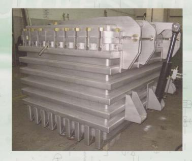
Ideal for cooking fruit of all sizes and extracting syrup by means of a dipping process.
