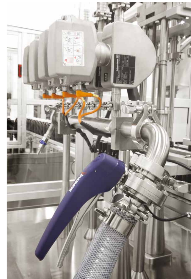
Valve to connect flow meters with lobe pump. Valvola di connessione tra massici e Pompa Lobi.
