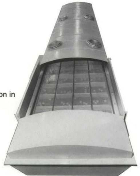
Channels separate rubber parts, convey to built-in water spray and air dry sections
