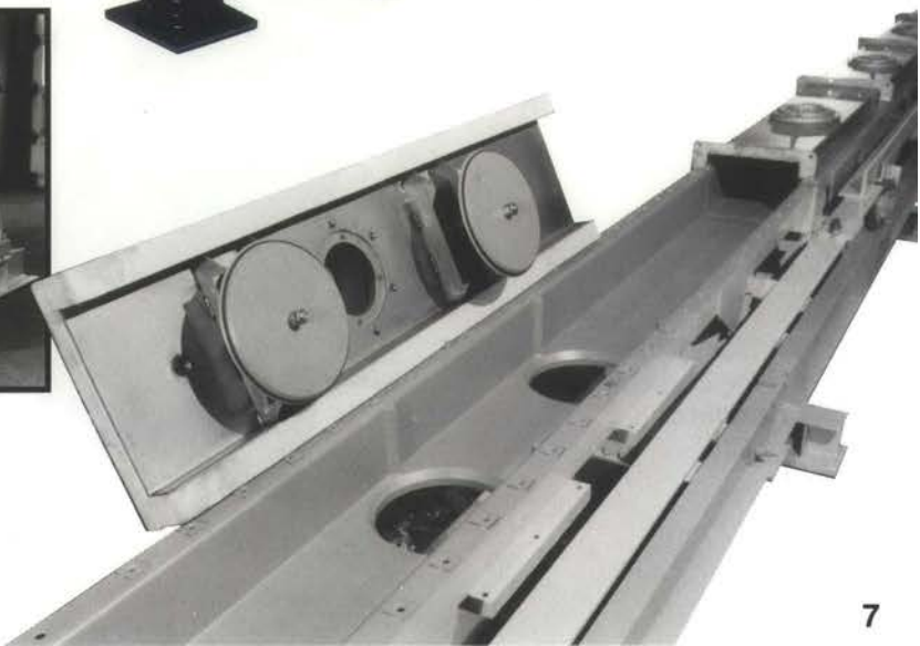
Air cylinder-operated gates divert prills
