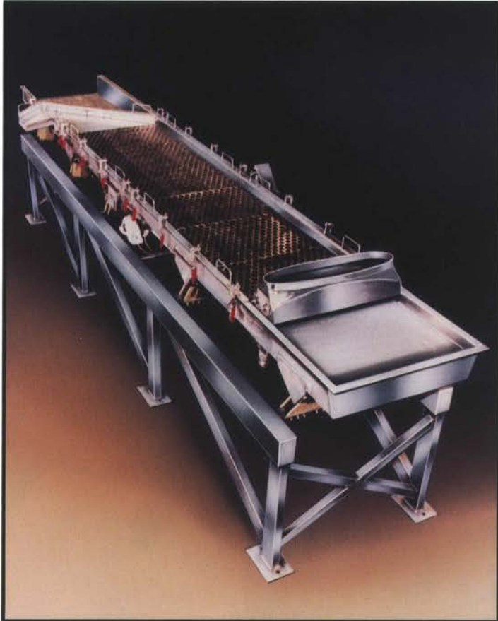
Meat pieces are sorted, classified, oriented and conveyed to packaging
