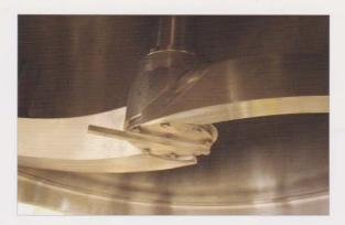
The agitator is internally heated for a better drying process and it can be operated at different speed, direction of rotation and height.
