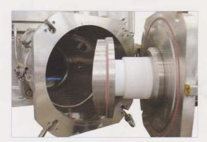
The side discharge valve has a particular conical shape that allows to minimize friction and dead volume.
