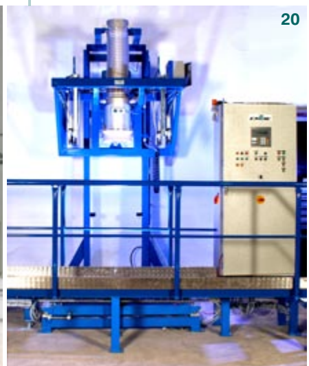
FIBC Filling Station with roller conveyor and operating platform
