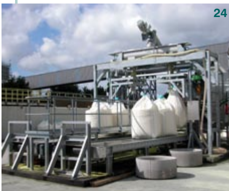
Double Filling Station for automatic filling in single-loop FIBCs
