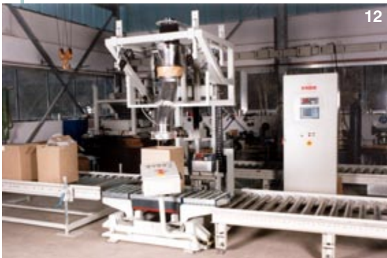
Composite station for cardboard and FIBCs in the food industry
