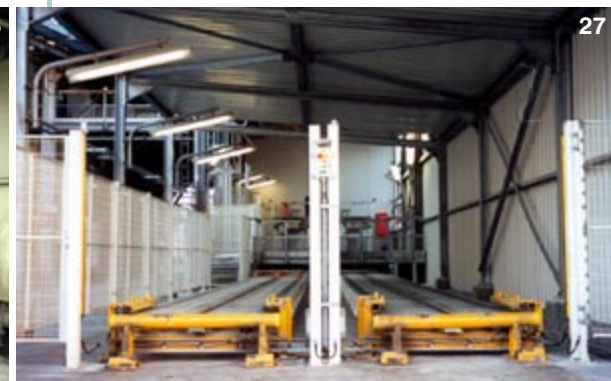
Discharging conveyor with handover point for fork lifts and safety technology
