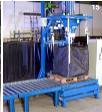
Filling Station with ground-frame integrated weighing system and accumulating roller conveyors
