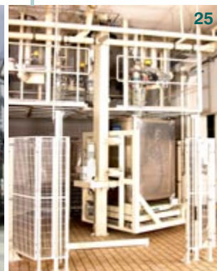
Filling carousel for IBC with integrated weighing system and dosing screw
