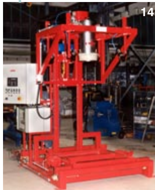
Compact Filling Station with flat vibration table for colouring pigments
