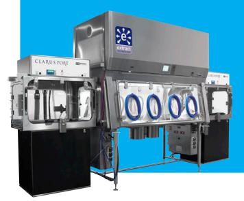
A uniquely designed supply/exhaust air system not only prevented cross contamination through each of the work stations but also created and maintained an EU Grade A (ISO5) environment without the need for external ducts or increasing the operating footprint. The integration of a gassing-in-place system the "Aseptic Hold" is based upon two weekly gassing cycles of the entire Isolator, securing material transfer with 6 log sporicidal decontamination steps at each load transfer via Clarus PORTS.
