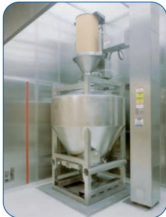
**IBC Charging using a Post Hoist**
