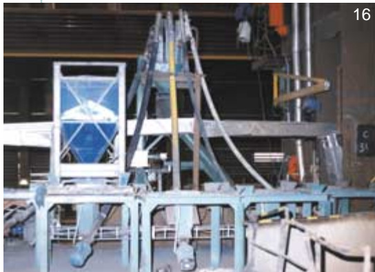
Dosing of alloys in a steel works with five EMDE-LIFT MDB 90 und MDB 70
