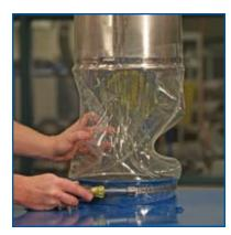
**3.** With the ROTEX PolyClear Sleeve gathered in that position, attach the free end to the bottom pipe and secure with a band clamp.
