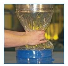
2. Gather the ROTEX PolyClear Sleeve around the circumference at the approximate middle of the connecting sleeve's length and squeeze the sleeve closed. The sleeve will resemble an hourglass shape.
