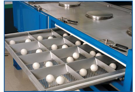
Balls reduce blinding of near-size material.
